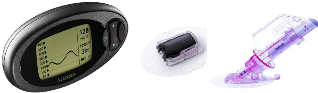
Figure 1.2 Components of the SEVEN® PLUS System: on the left the Receiver, a cell-phone sized device programmed to collect and process data from the sensor and to display the results as a glucose values, in the middle the Sensor with the Transmitter, on the right the Sensor with the applicator, used to insert the probe underneath the skin.
