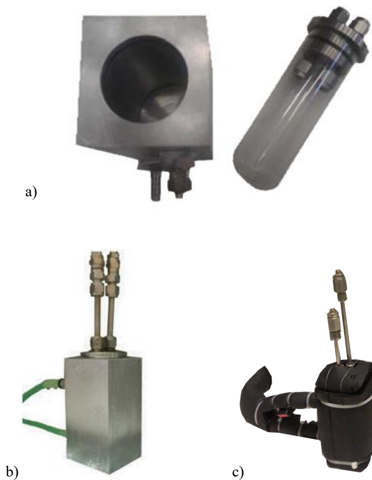
Figure 3.8 Details of the condenser that was used to remove water in the gas leaving the reactor: a) the aluminium body and the glass tube; b) the aluminium body with two connectors for the inlet and the outlet of the cooling fluid; c) insulating material cover that minimizes energy losses due to heat exchange.
