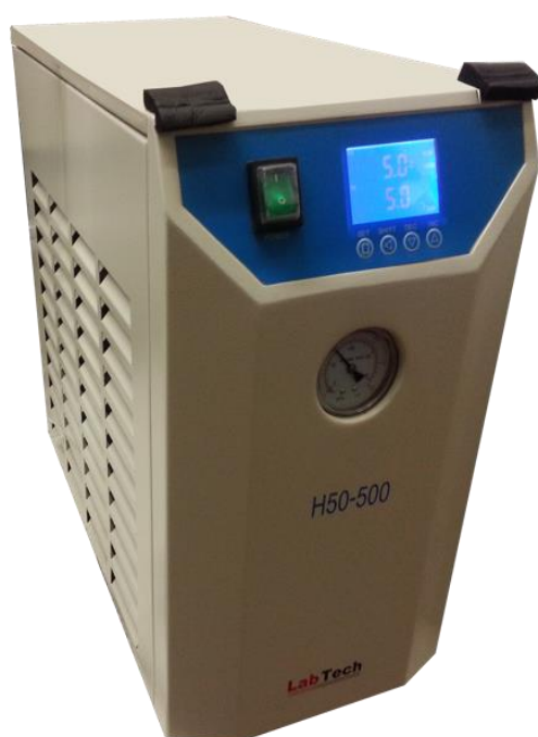
Figure 3.7 Chiller used to maintain the temperature of cooling fluid at setpoint
