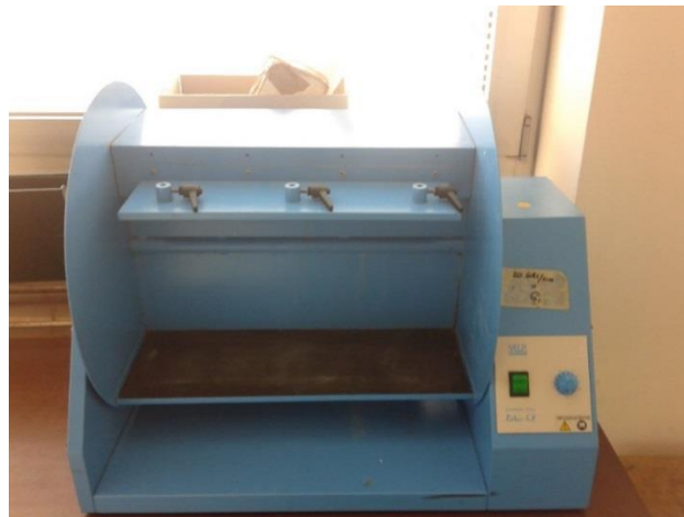
Figure 3.23: Agitating machine. The equipment has 6 place, three visible and three in the opposite side, at which bottles are attached. In bottles the water and the sample are continuously turned by the machine to extract all possible compounds. The turning rate is 20 rounds per minute, for 24 hours.
