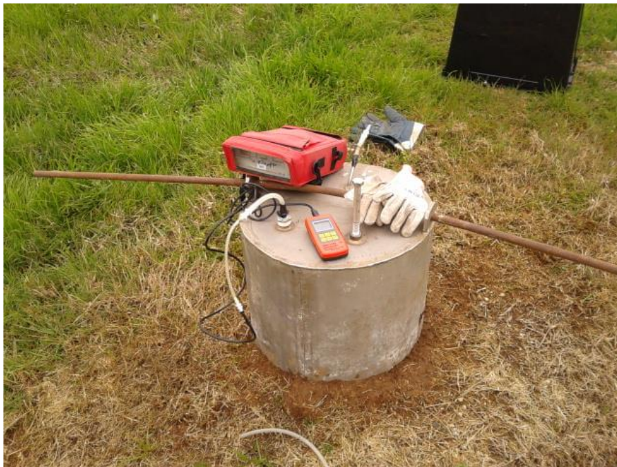
Figure 3.26 Static chamber equipment planted in soil, connected with the LFG20 (red instrument) for the concentration of oxygen, carbon dioxide and methane and with the pressure probe (orange instrument) for the pressure monitoring.
