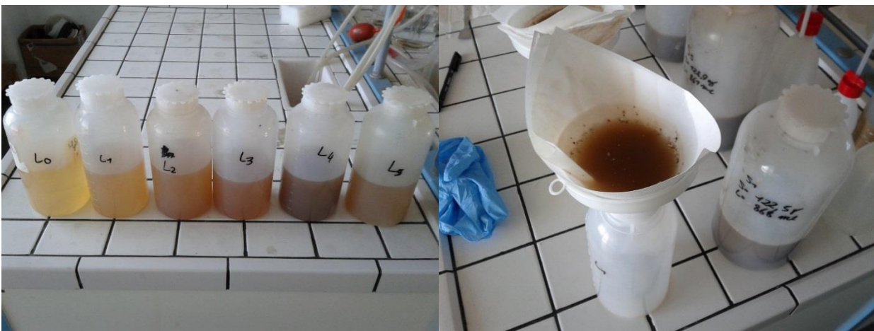
Figure 3.24: Leaching test result. A: final eluate extract by leaching test, more or less 500 ml per sample. B: Filtering process with filter paper, the process requires a lot of time because the high turbidity of the samples.
