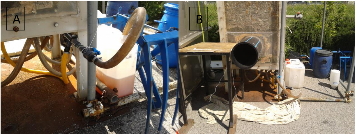
Figure 1.7: Lysimeter of the ICEA department in “Voltabarozzo” Padova University. A: Particular of the leachate collection system under the bottom of the reactor and of the canisters used for the collection. B: Frontal view of the equipment with the leachate collection system and the natural aeration HDPE tube.
