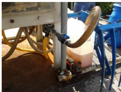
Figure 3.25: Lysimeter leachate collection system. The structure on the left is the lysimeter. The rubber pipes on the left come from the bottom of the reactor, and reach the plastic pipe in the center of the figure. From the plastic pipe, another rubber tube reaches the canister on the right. The flux can be managed with the blue valve. The system is always in pressure because of the low space for tanks under the reactor.
