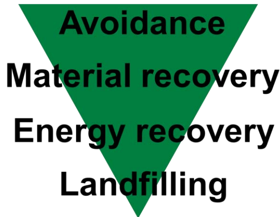
Figure 1.3: Pyramidal policy for waste management in Europe. First avoidance, second material recover, third energy recover, fourth landfilling.
