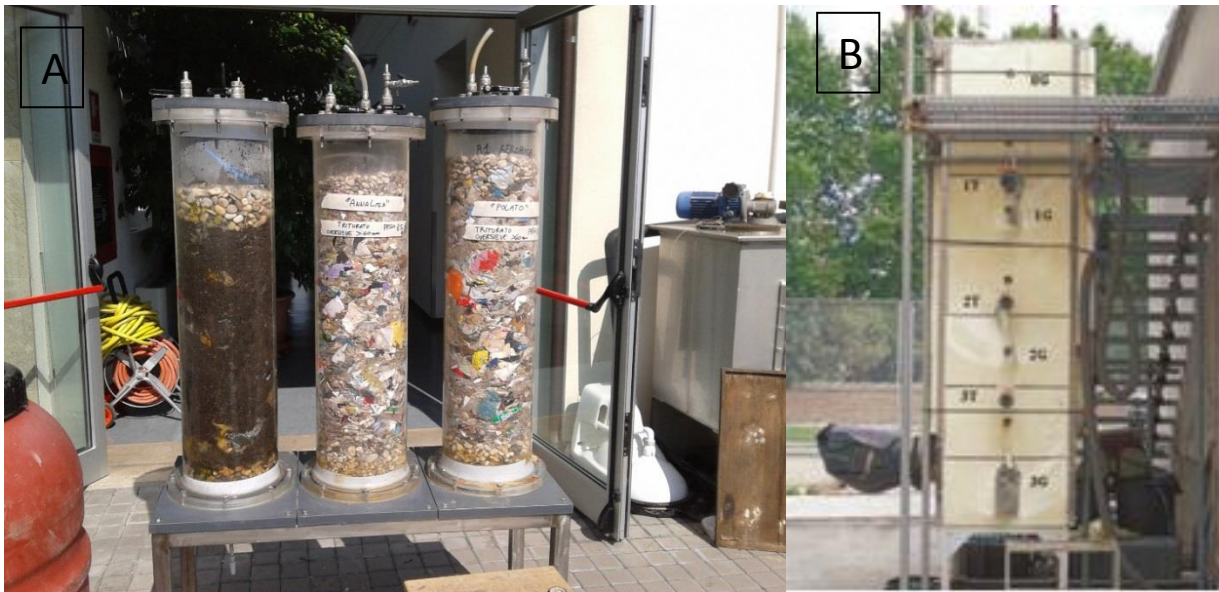
Figure 1.5: A: Columnar tests, these columns are in the ICEA department in “Voltabarozzo” Padova University. The left one are old foundry soils, the other two are fresh over-sieve >60 mm waste just putted in. These columns are high one meter, gas valves for leachate under the bottom and systems for water and air controlled circulation, can be completely filled of water and can be cover with a thermic blanket for set a temperature. Their capacity vary from 5 to 50 Kg depending on density. Gravel are dispose on the bottom and on the top of the sample to enhance the circulation of fluids. B: Lysimeter test, this reactor is in the ICEA department in “Voltabarozzo” Padova University too. This equipment is the same used in this thesis, the image is take in 2005 during the first phase of anaerobic treatment. The description of the is in the following chapter.
