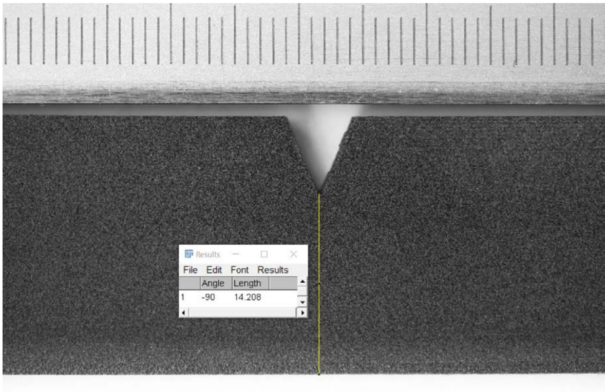
Figure G.18: Measure of the net width of the 90VR0PA12_-1_1BIS specimen.
