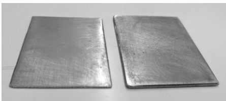
Figure 3.2.2.2: View of the two types of slat that have been used. On the left there is the 0,5 mm thick one and, on the right, there is the 1,5 mm thick one.
