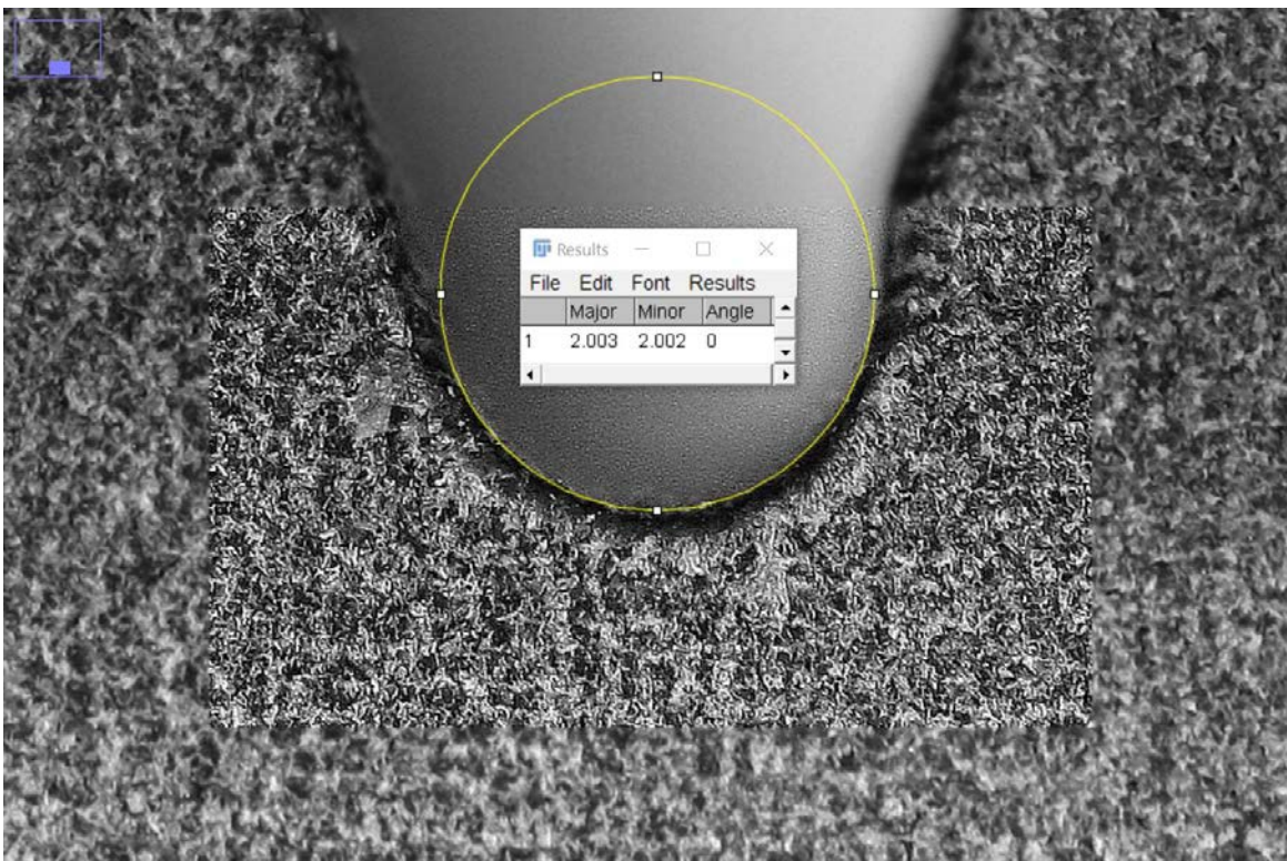
Figure F.36: Measure of the V-notch apex diameter of the 90VR1PA12_-1_11 specimen.
