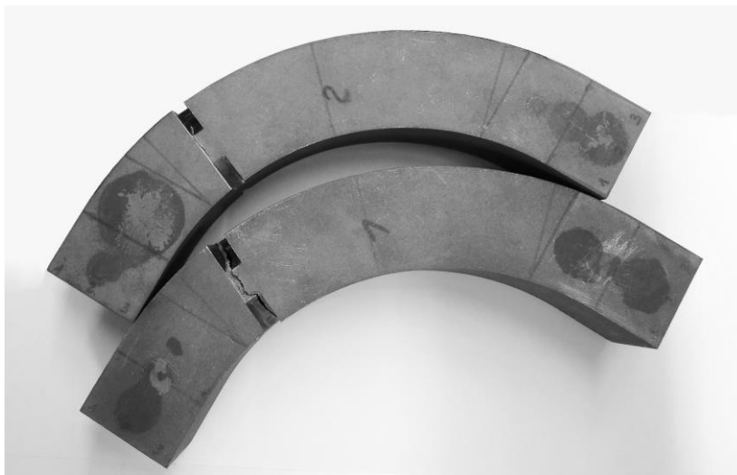
Figure 3.2.3.8: Maraging steel curved beams, number 1 and number 2, broken after the static tests.
