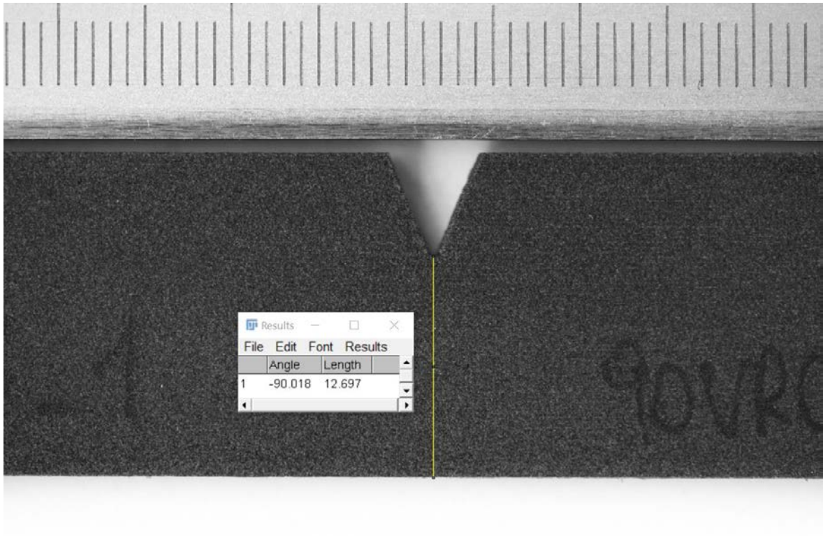
Figure G.17: Measure of the net width of the 90VR0PA12_-1_1 specimen.
