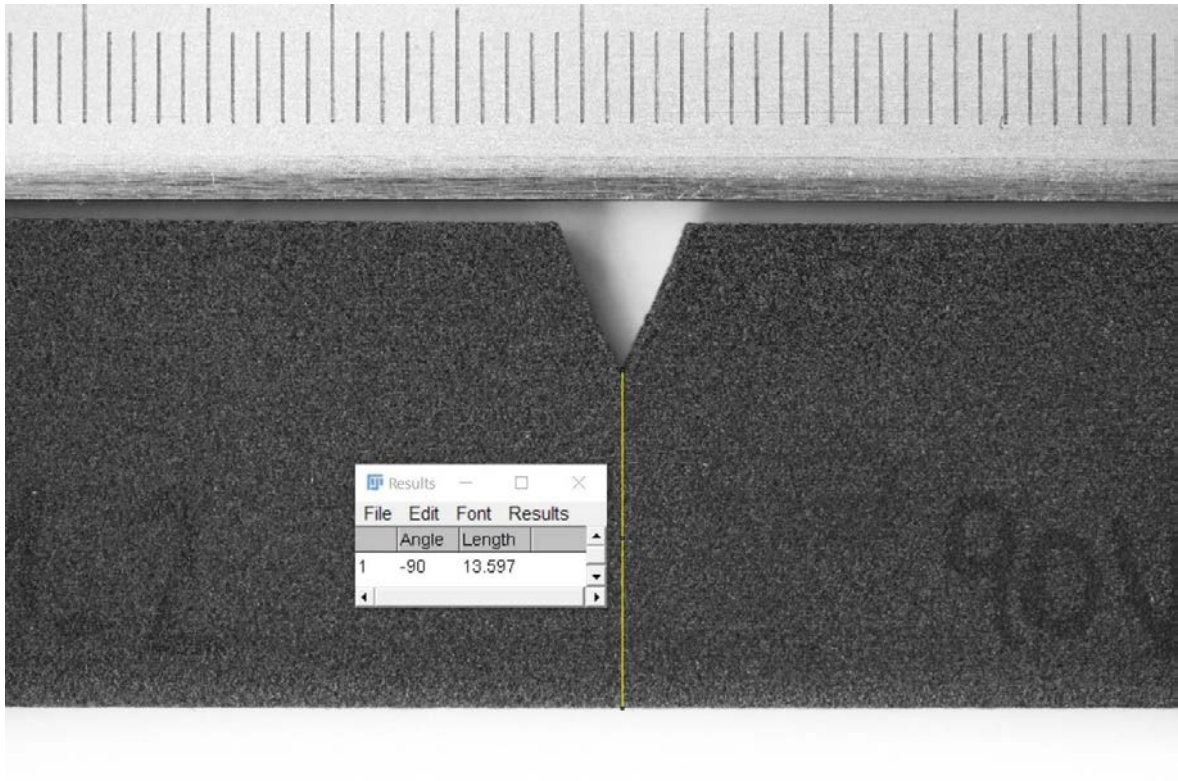
Figure G.19: Measure of the net width of the 90VR0PA12_-1_2 specimen.
