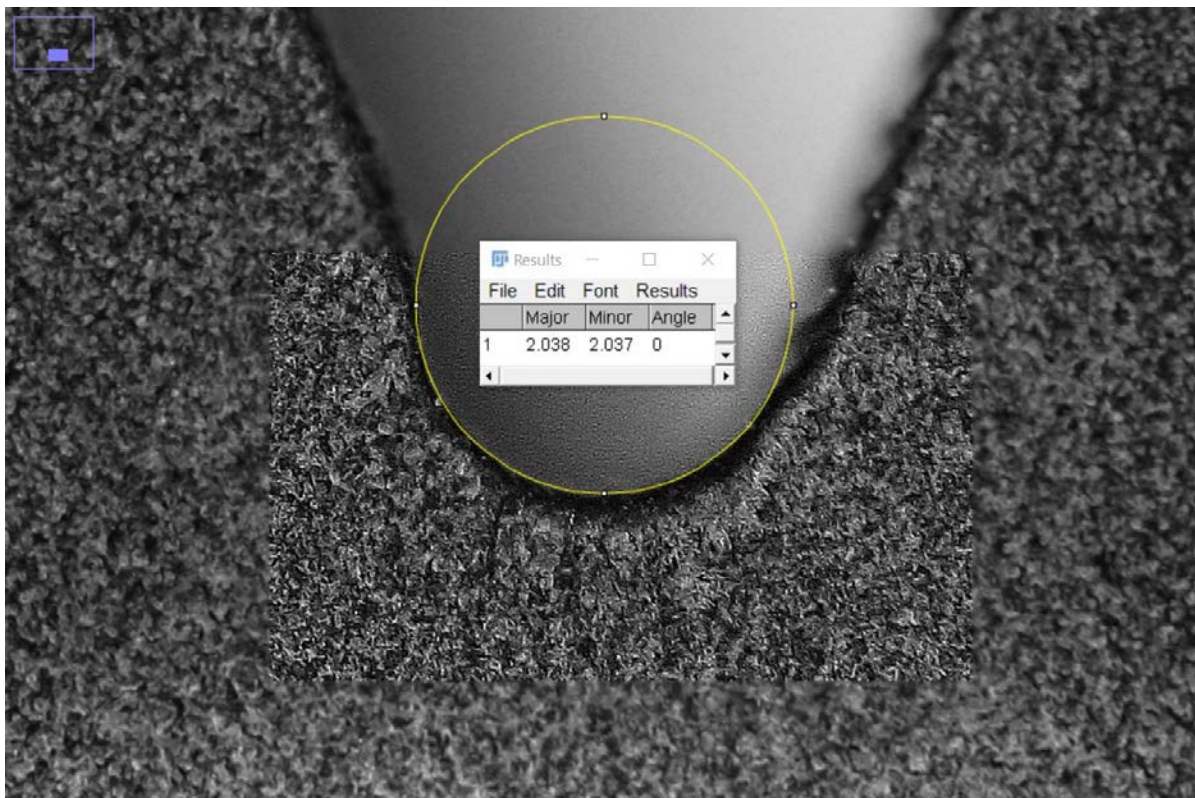
Figure F.20: Measure of the V-notch apex diameter of the 45VR1PA12_-1_7 specimen.
