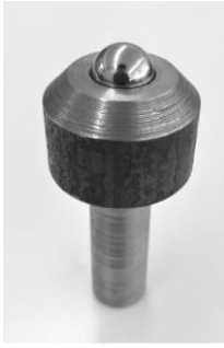
Figure 3.2.2.3: View of the custom made tool with the bearing ball.
