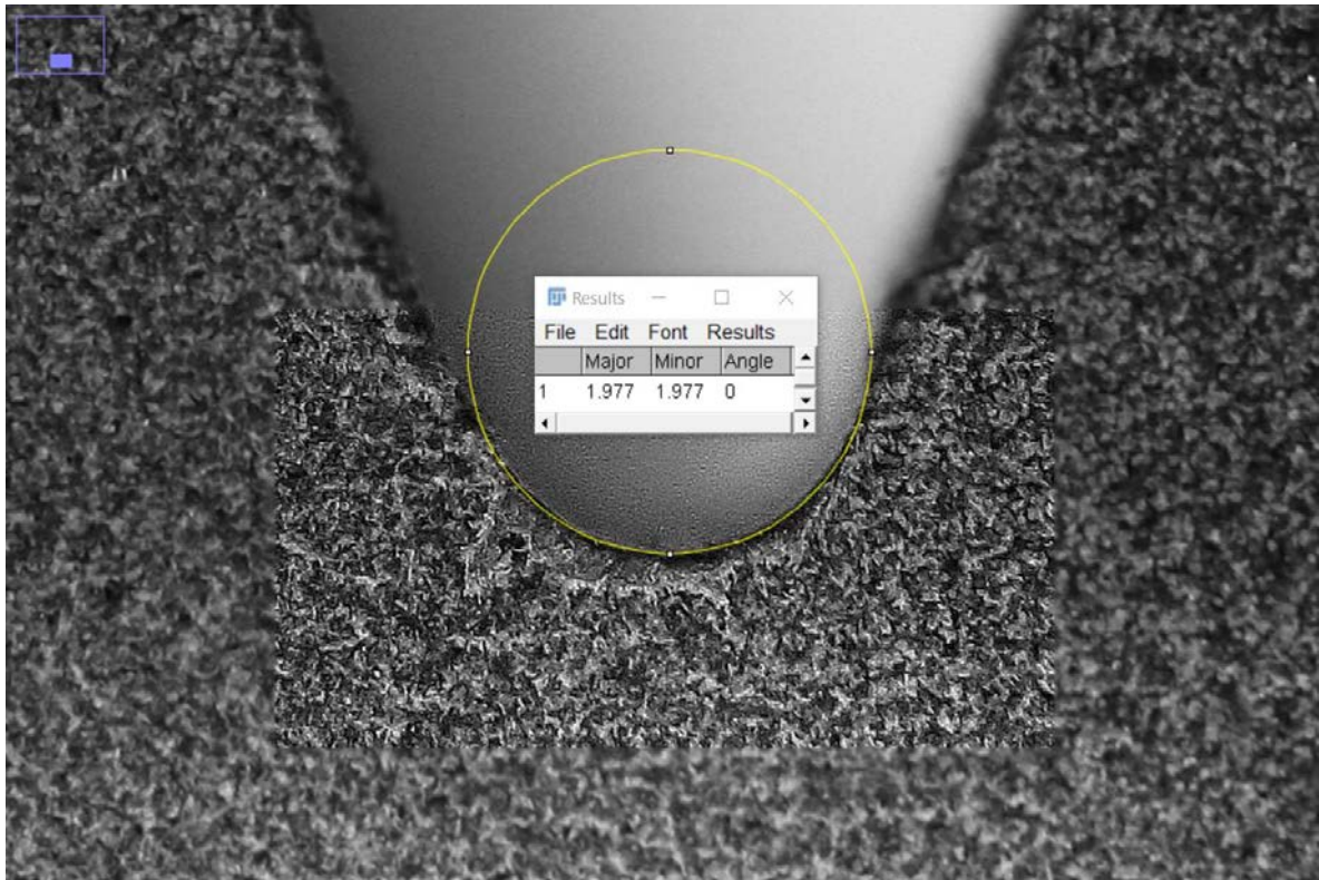
Figure F.31: Measure of the V-notch apex diameter of the 90VR1PA12_-1_6 specimen.
