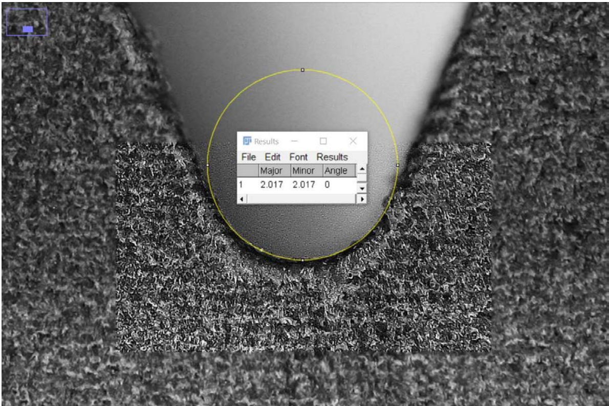
Figure F.28: Measure of the V-notch apex diameter of the 90VR1PA12_-1_3 specimen.
