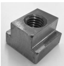
Figure 3.1.2.8: Special nut for bolting the Base part to the MTS 25 kN table.
