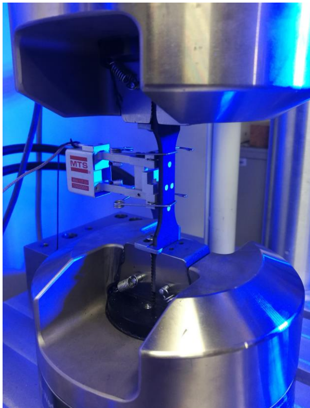
Figure 4.2.2.2: Mechanical extensometer fixed to the specimen.
