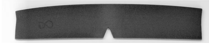
Figure 4.4.1.9: View of the 90VR1PA12_-1_8 specimen before the straightening procedure.
