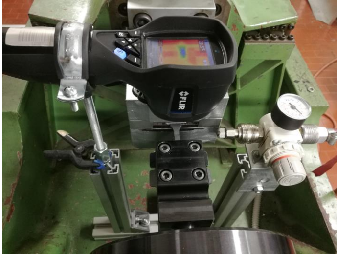
Figure 4.3.2.2: View of the prepared set-up for the fatigue tests of the PA12 specimens. It is possible to see a plain specimens clamped, the FLIR thermal imaging camera that has been used to monitor the specimen's temperature, the nozzle, connected to the compressed air circuit of the laboratory, that has been used to blow fresh air to the specimens.
