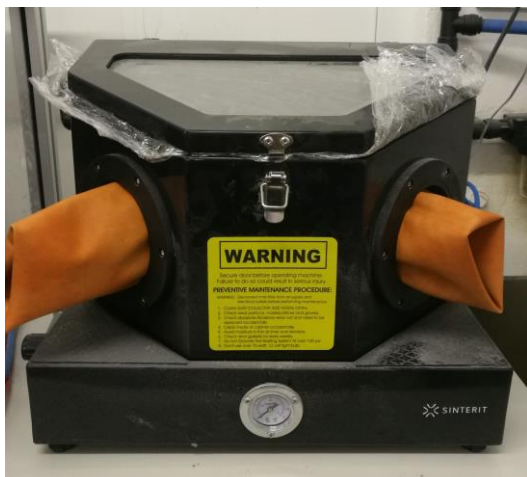
Figure 4.1.5: View of the “Sinterit” sandblaster.
