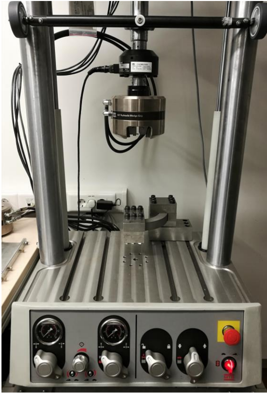
Figure 3.2.2.1: View of the 25 kN MTS test machine with the lower grip removed and with the Maraging steel clamps set - up.
