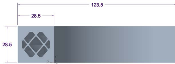
Figure 3.2.1.3: XY-plane view of the PA12 curved beam with the structural inner support developed in Subchapter 2.5.7 (mm).
