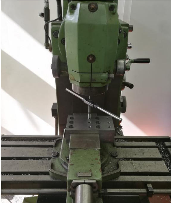
Figure 3.1.2.1: View of the central part of the three axis milling machine. It is possible to see also the Base part during the holes threading process.
