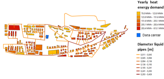
Figure 4.8: District design with the data center (vapour)
