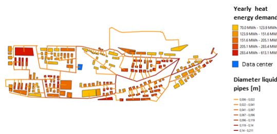
Figure 4.7: District design with the data center (liquid)
