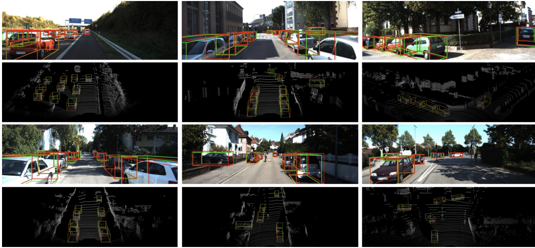
Figure 1.1: 3D Object detection task in the automotive environment from CIA-SSD [15] paper
