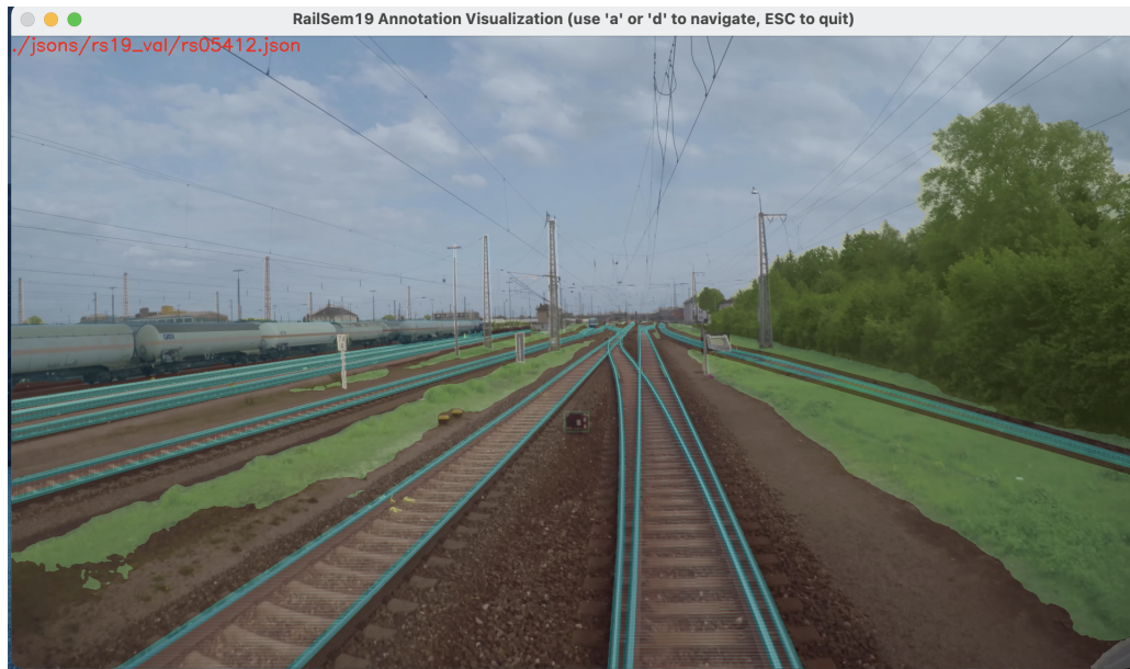
Figure 2.6: Example of image with semantic segmentation and object detection labels.
