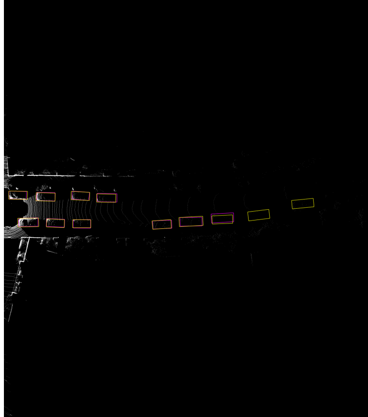
Figure 5.2: Example of successful car detection on KITTI dataset using VoxelNet on bird view . Purple is the ground truth whereas yellow is the network prediction.
