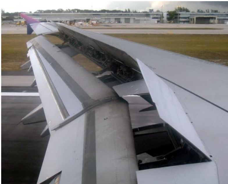
Figure 1.6. Conventional spoilers in action during landing brake on the ground: the large deflection increases drag force which is useful to help the undercarriage brakes.
