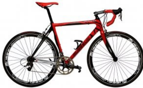
Figure 3.19 The Belgian framemaker Museeuw has been creating a new carbon hybrid composite made up by flax fibers and ultramodern carbon fibers. The new material is thought to have exceptional shock adsorbing capabilities, demonstrating how flax fibers can be useful also as further reinforcement in already existing high performance composites [19].
