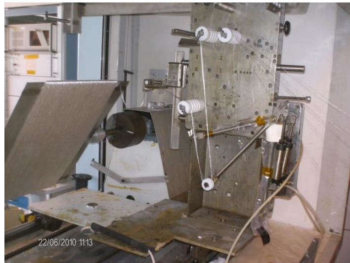
Figure 4.5 Example of filament winding operations.
