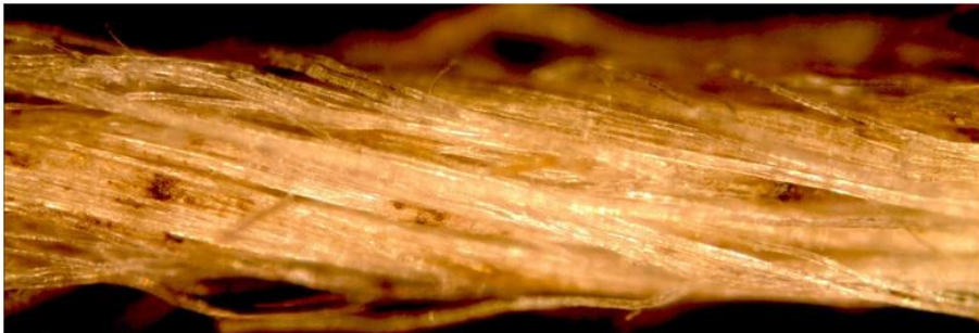
Figure 4.1 Example of neat flax yarn.
