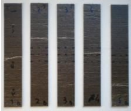
Twisted flax/PET, off-axis angle 90°
