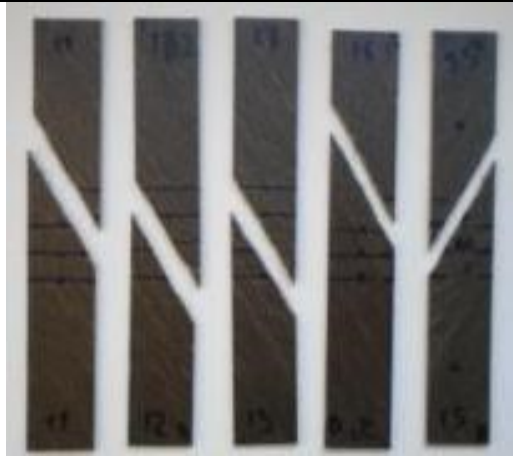
Twisted flax/PET, off-axis angle 30°
