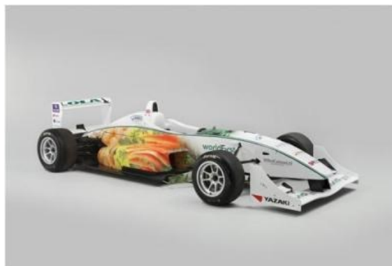
Figure 3.17 “World first formula 3 car” represents one of the most interesting application of biocomposite and recycled materials [17].
