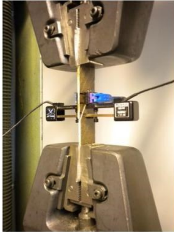
Figure 5.3 Tensile specimen mounted for testing with the two extensometers centred at the gauge section.
