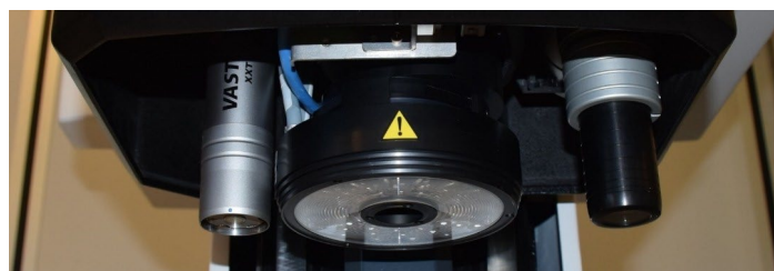
Figure 44. Zeiss O-Inspect 3/2/2 measuring head. From left to right: contact measuring probe housing, telecentric camera with illumination system, and confocal chromatic sensor.
