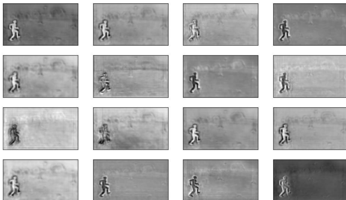
Fig. 3.18: 3 \times 3 convolutional layer after Spatial Dropout (64 feature maps of resolution 128 \times 72 )
