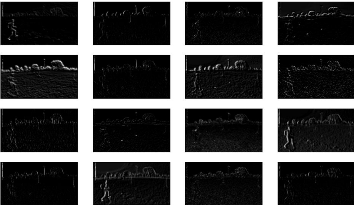
Fig. 3.5: Second convolutional layer of the second block (128 feature maps of resolution 256 \times 144 )
