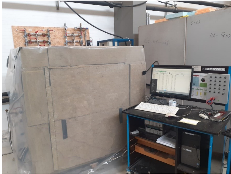
Figure 20: working desk with data acquisition system.
