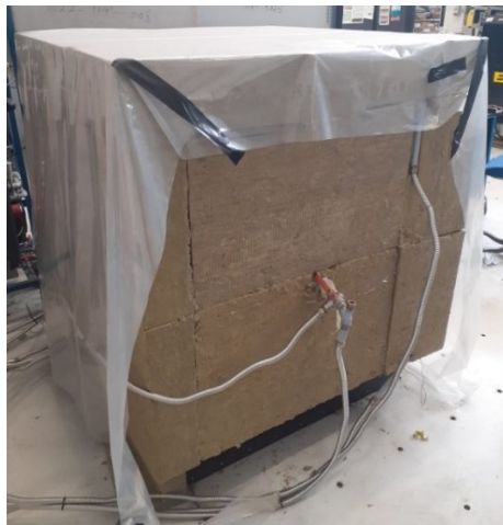
Figure 17: Coolant valve (top left), electric boiler (top right), soil box with insulation and pipes (bottom).
