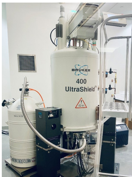
Figure 2.1: 400 MHz Avance NEO Bruker Spectrometer equip- ped with a BBI probe at the NMR Expertise Centre at Ghent University.
