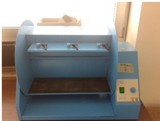
Figure 3.15: Agitating machine. The equipment has 6 place, three visible and three in the opposite side, at which bottles are attached. In bottles the water and the sample are continuously turned by the machine to extract all possible compounds. The turning rate is 20 rounds per minute, for 24 hours.
