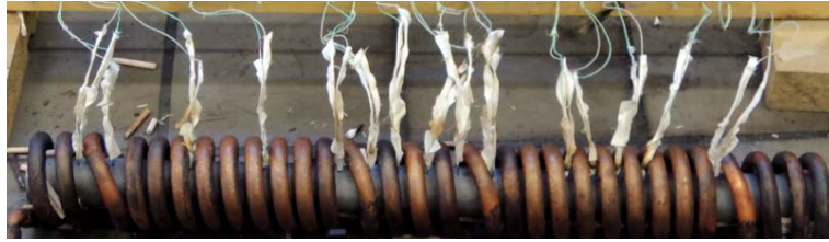
Figure 4.15. Thermocouples and Teflon tape insulation
