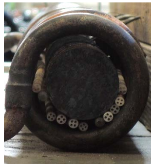
Figure 4.13. Ceramic tubes keep the work-piece at the centre of the inductor
