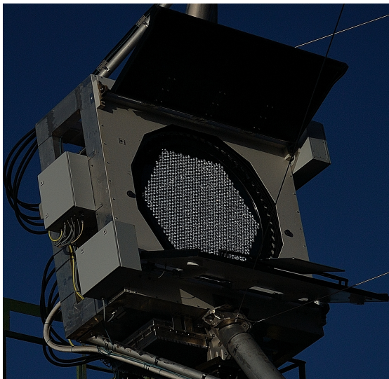
Figure 2.15: Camera of MAGIC-I. The picture was taken in daylight with the lids closed since the electronics were shut down.
