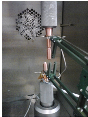
Figure 4.10: Broken specimen with notch acuity 2 on the NT101 machine
