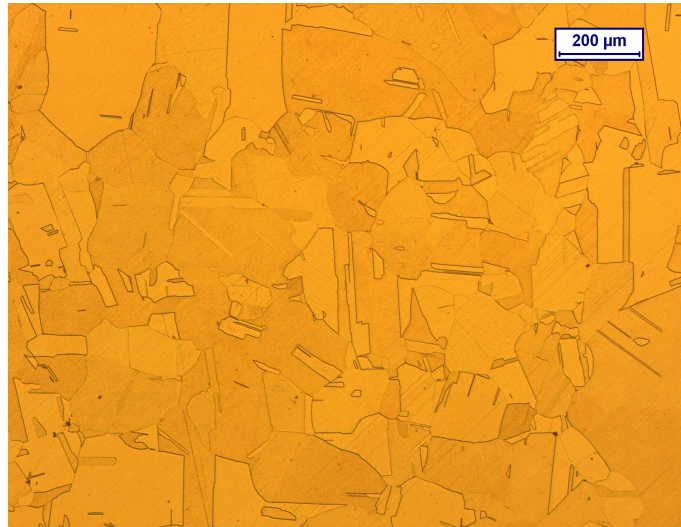
Figure 5.50: Specimen 43, not tested. The specimen's original microstructure shows mixed grains size and orientation.
