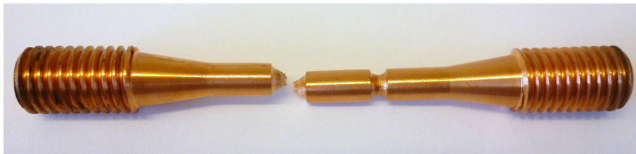
Figure 4.11: Broken specimen with acuity 2, exposed to \dot{\epsilon} = 10^{-6}s^{-1} and T=75^{\circ}C
