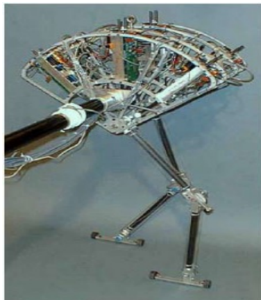
Figure 3.3: Spring Flamingo: walking robot that employ Series Elastic Actuators
