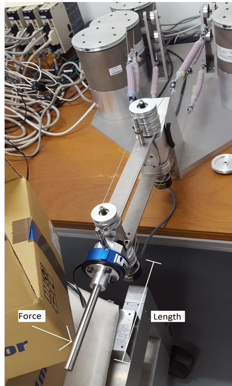
Figure 5.3: Force measurement by using force sensor
