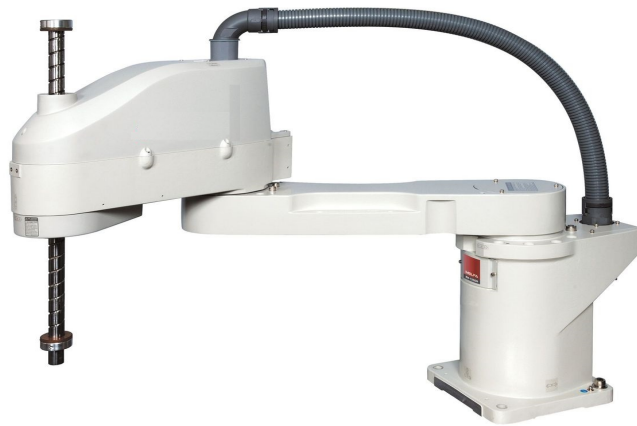
Figure 1.1: rigid robot: SCARA
