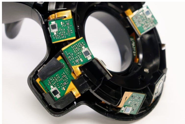
Figure 6: portion of the Vive's controller ring. 9
