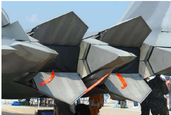
Figure 7: The 2D MLN rectangular nozzle of the F-22 Raptor [9]
