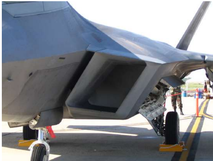
Figure 9: The Caret inlets particular of a F-22 Raptor [9]
