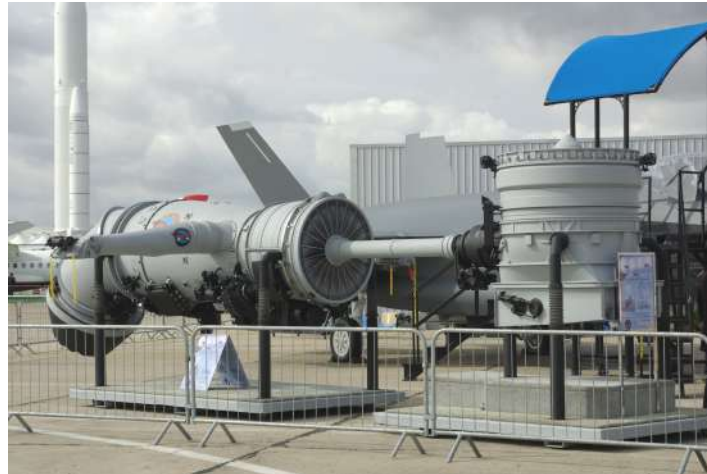
Figure 11: F-135-PW-600, the VTOL version with the lift fan [14]
