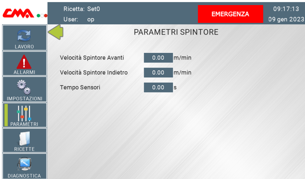
Figure 3.25: Parameter page of the Cart-Pusher station
