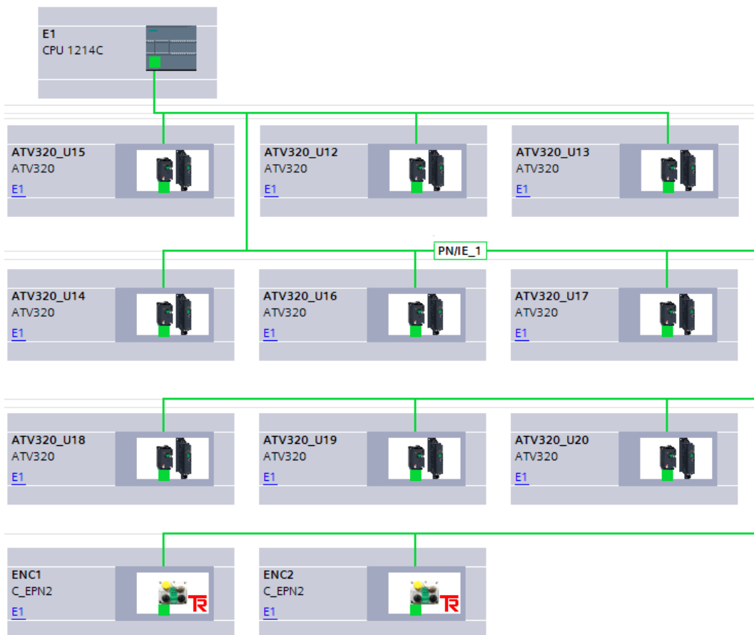
Figure 1.16: Layout of the PROFINET network
