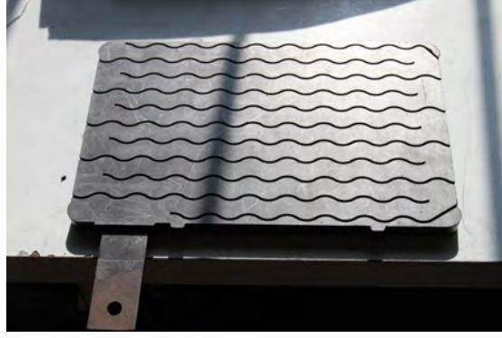
Figure 3.5: Monopolar plate with interdigitated channels
