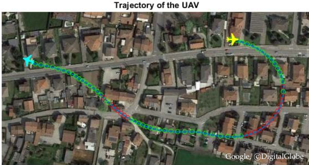
Figure 76.: Trajectory of the UAV in a city centre, i.e. in an area of high complexity; the red dots represent the time instants in which a re-allocation of resources happens.
