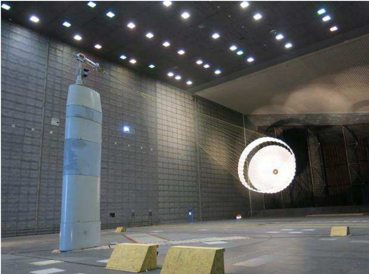
Figure 1.3: Schiaparelli DGB parachute during testing [3].
