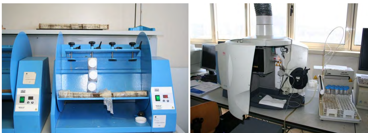
Fig. 7.5.2.1 Water leaching test and ICP analysis.
