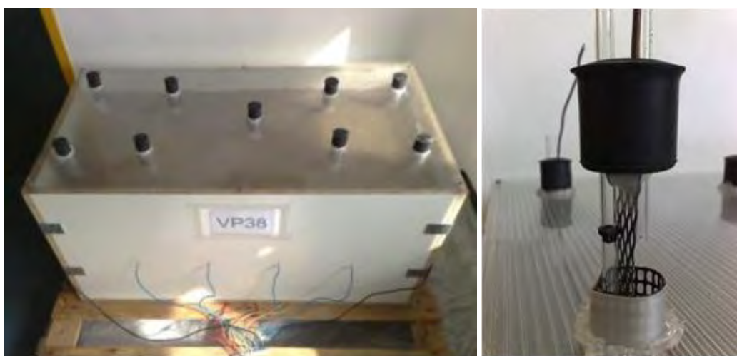
Fig. 7.2.1.2 Setup of the bench-scale ECRT and particular of activated titanium electrode.
