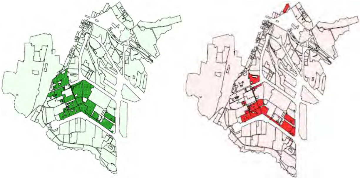
Fig. 4.5.2 ■ areas planned for MPE/TPE treatment, ■ areas planned for SVE treatment. Source: D'Aprile, 2007 .
