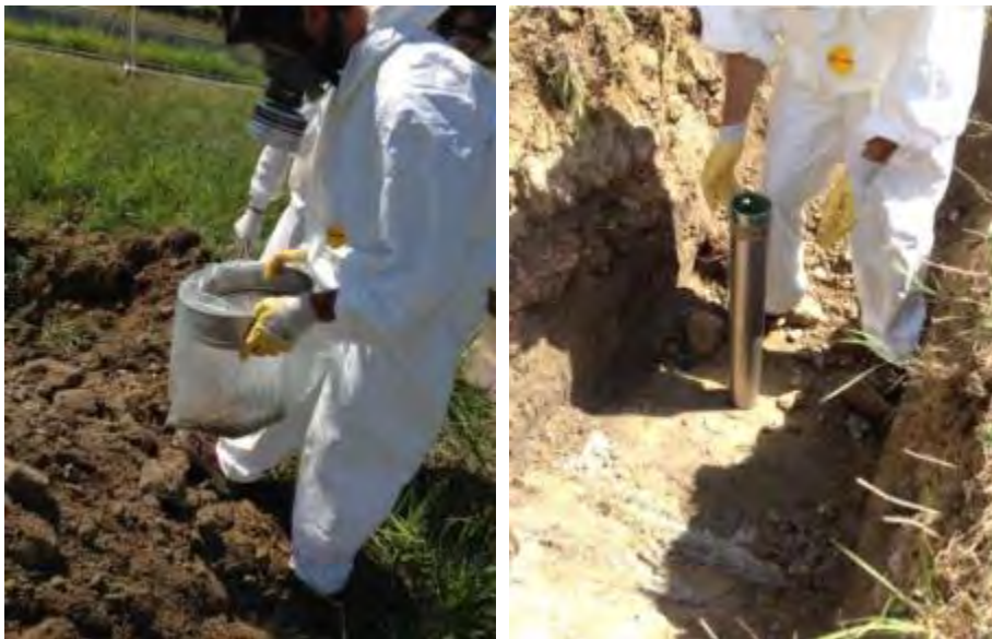
Fig. 7.7.1.3 Extracted soil sampling and samples extraction by probing .
