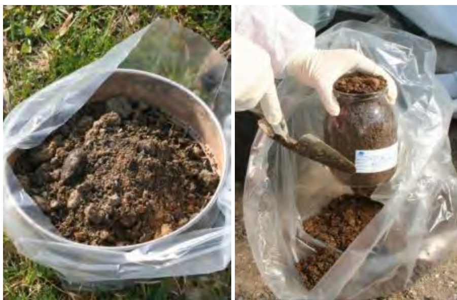
Fig. 7.7.2.6 Soil sieving at 2cm and sample storage in glass bins.
