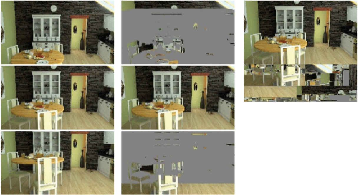
Figure 3.18: Input views in the left, views after pruning in the middle, atlas in the right
