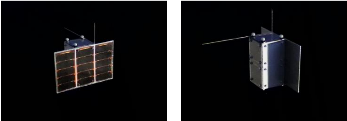
Figure 4.2 Back and front face of the CubeSat model with the main solar panel, two antennas and three IR reflective markers on the top surface.
