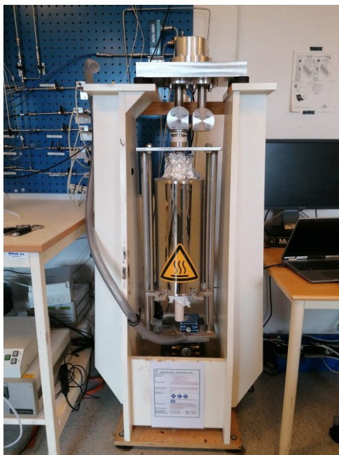
Fig. 3.6 Picture of the home-made thermogravimetric instrumentation.
