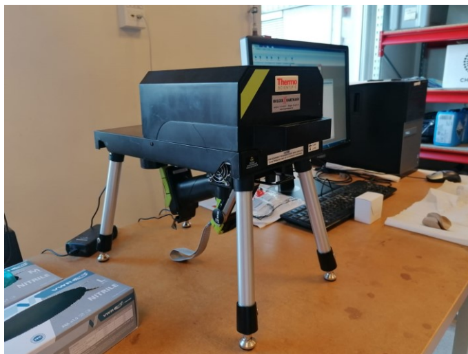
Fig. 3.2 Picture of Niton XL5 Plus portable instrument.
