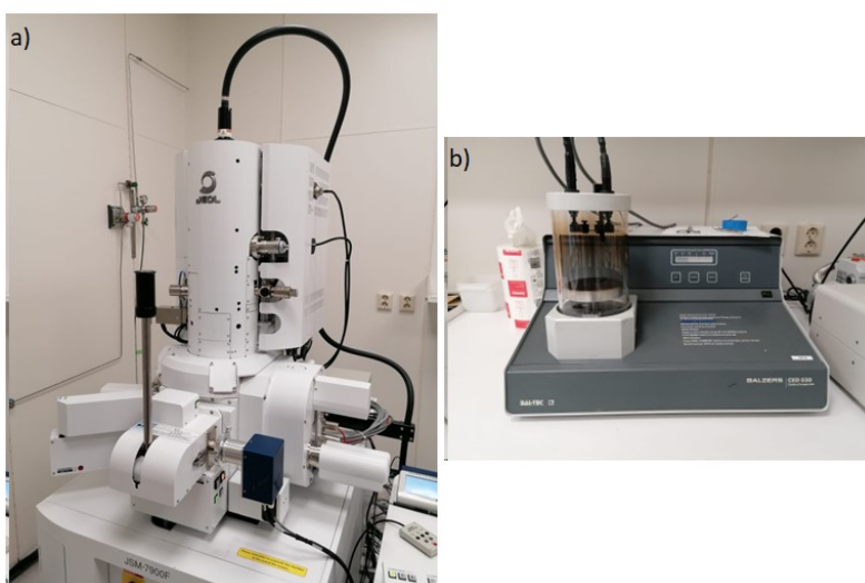
Fig. 3.7 Pictures of a) JSM-7900F electron microscope and of b) CED 030 Balzers carbon evaporator.
