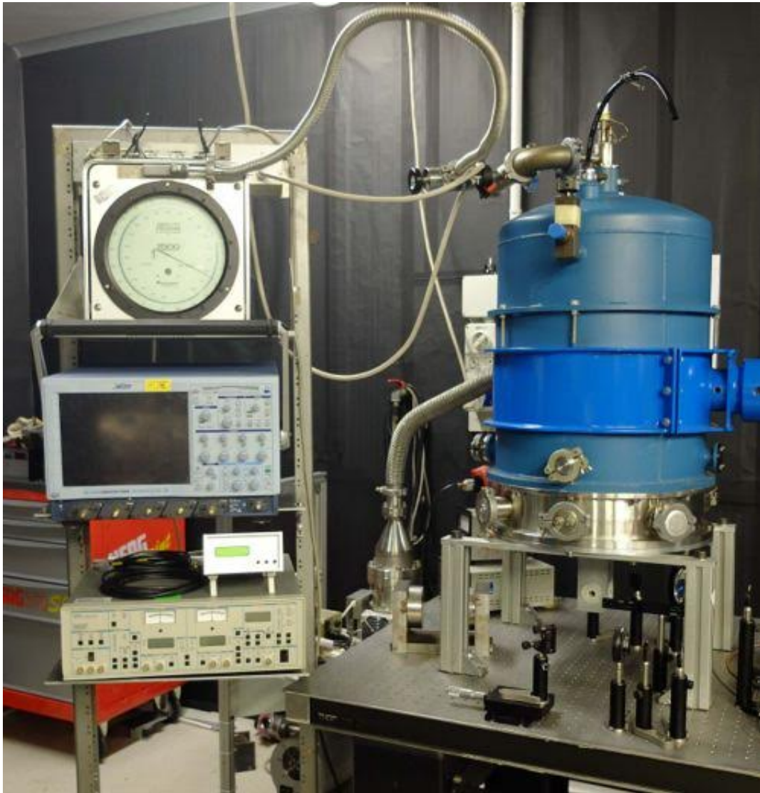
Figure 3.1: Cryogenic and measurement parts of the experimental setup; the window under the cryostat is where the crystal is located during the experiment.
