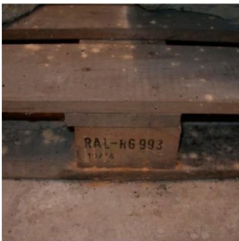
Figure 8 Pallet infested by wood borer beetles; the holes on the wood are visible signs of infestation (Source: Biebl, S. and Querner, P., 2020, photo by P. Querner)
