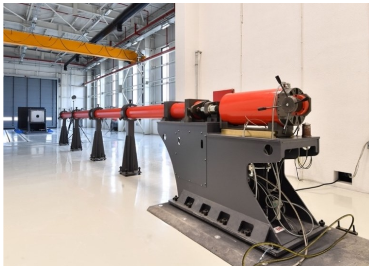
Figura 1.13: tipico ambiente di lavoro per i test sul bird strike. [“TAI builds Turkey’s 1st bird strike testing facility for aircraft” (2022). www.dailysabah.com ]
