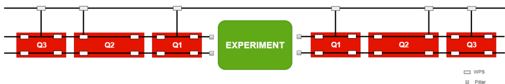
Figure 12: WPS sensors in the LSS
