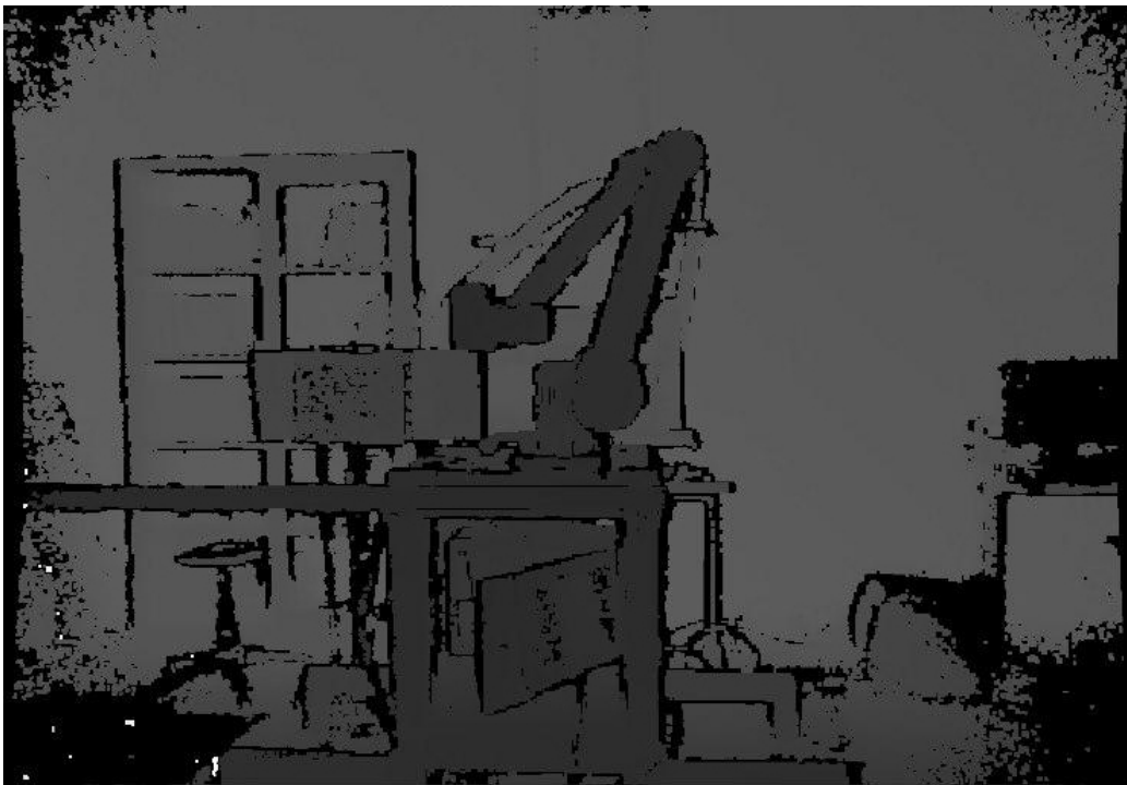
Figure 5.7: A depth map from the Kinect v2 sensor.
