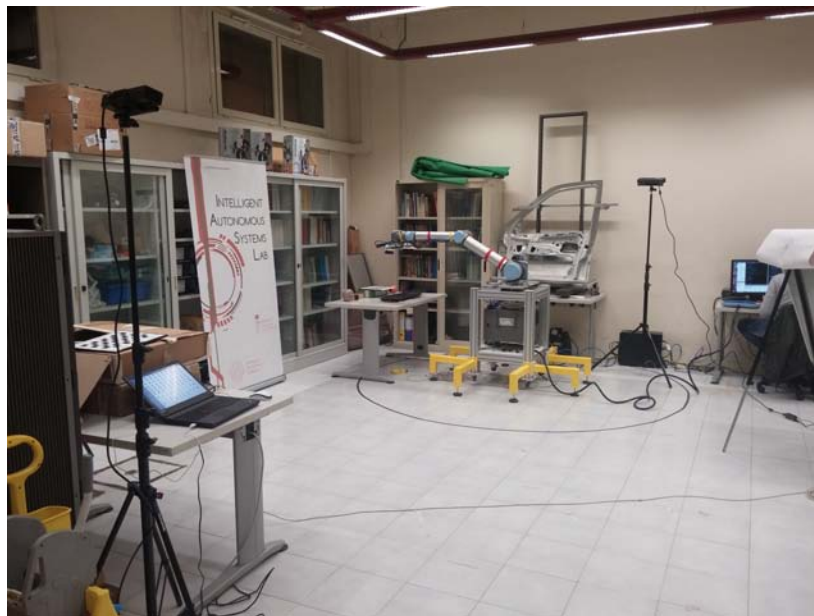
Figure 11: The IASLab setup, the camera in the foreground at the left is connected to the master node while the kinect on the right is linked to the “client” node
