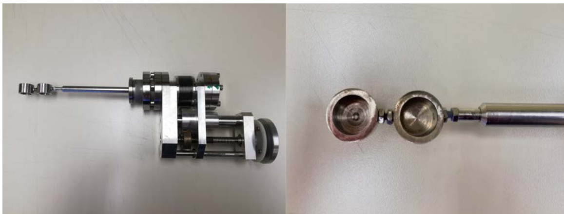
Figure 4.8: a) Collectors mounted in a manipulator; b) the two movable collector: the right one blank and the left one with a 1.8 mm hole
