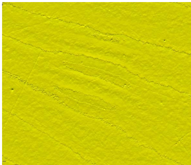
Figure 5.1: Image taken with the profilometer. S_a=3.3 nm
