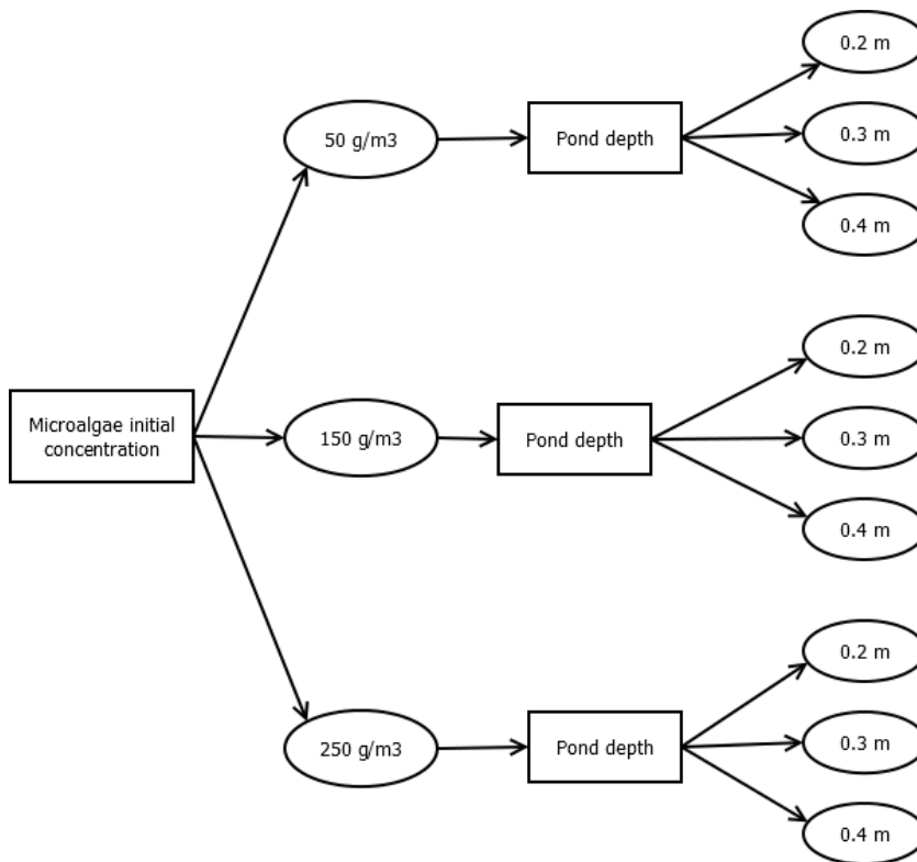
Figure 15: Simulation tree for open pond parametric analysis
