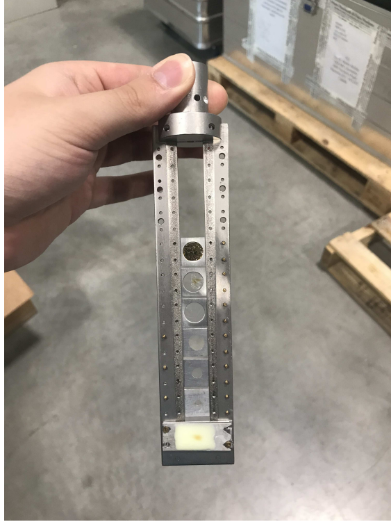
Figure 4.4: The target holder used in the experiment: as it can be seen, there are different types of target used throughout the experimental run. From above: a thin foil of pure ^{197}\text{Au} ( 90 \mu\text{g}/\text{cm}^2 ), two targets of \text{CD}_2 with a thickness of 116 \mu\text{g}/\text{cm}^2 , three “collimators” (anti-scattering diaphragms) of respectively 4.7 - 2.5 - 2 mm of diameter. The last step is a ZnS layer in which we can see the beam spot in dark yellow.
