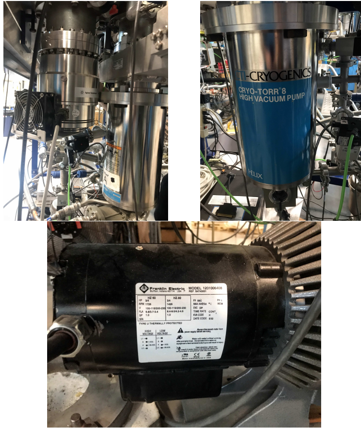
Figure 4.11: Photo of the vacuum pumps used in the laboratory: from top to bottom, left to right, there are the TMP, the cryogenic pump and the rotary vane pump.
