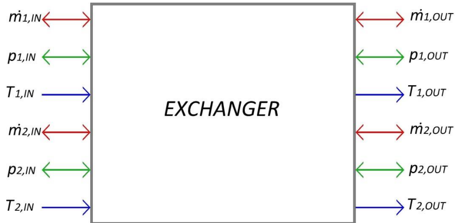
Figure 3.3 Causality diagram of heat exchanger dynamic model.
