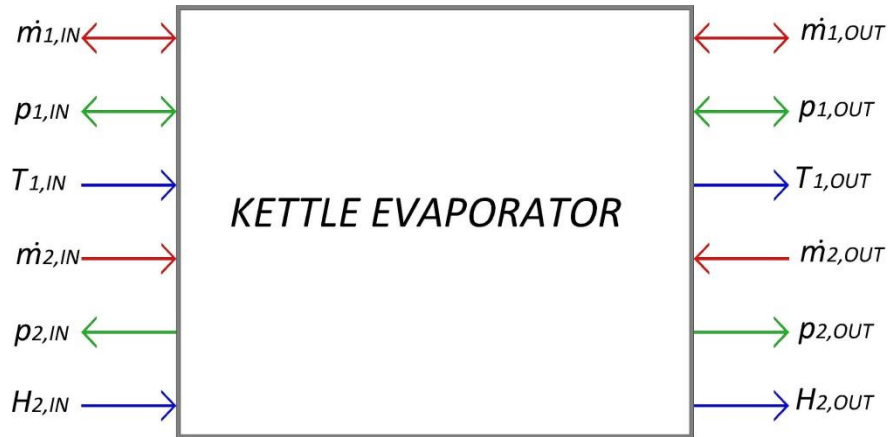
Figure 3.6 Causality diagram of evaporator dynamic model.
