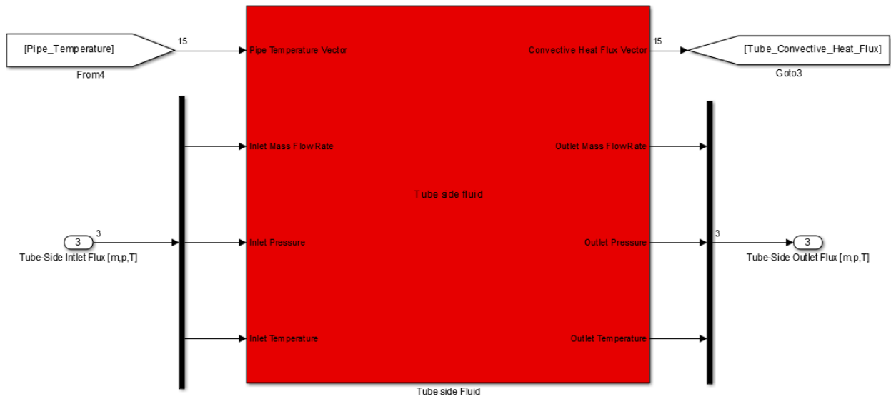
Fig. A2. 55 Block diagram of Tube side fluid subsystem, Kettle evaporator, (level 3 of hierarchy)
