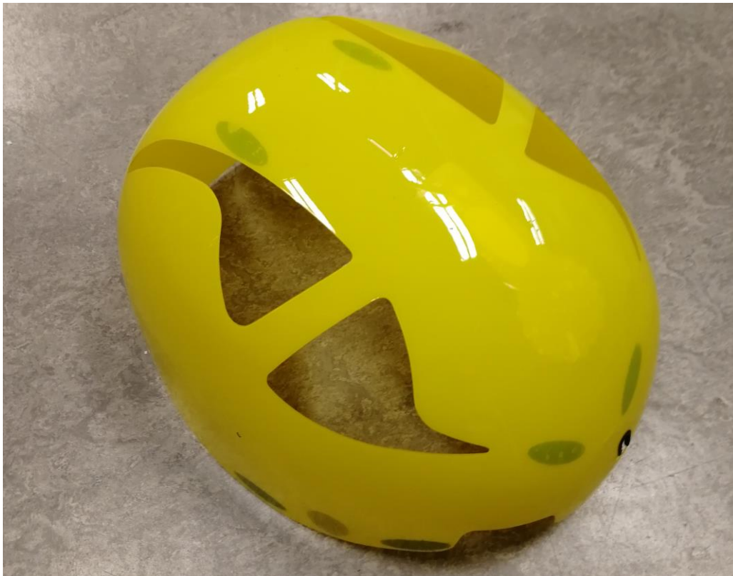
Figure 5.7 Low friction layer posed between the external protection shell and the internal energy-absorbing polymer foam liner of the MIPS helmet used during tests.
