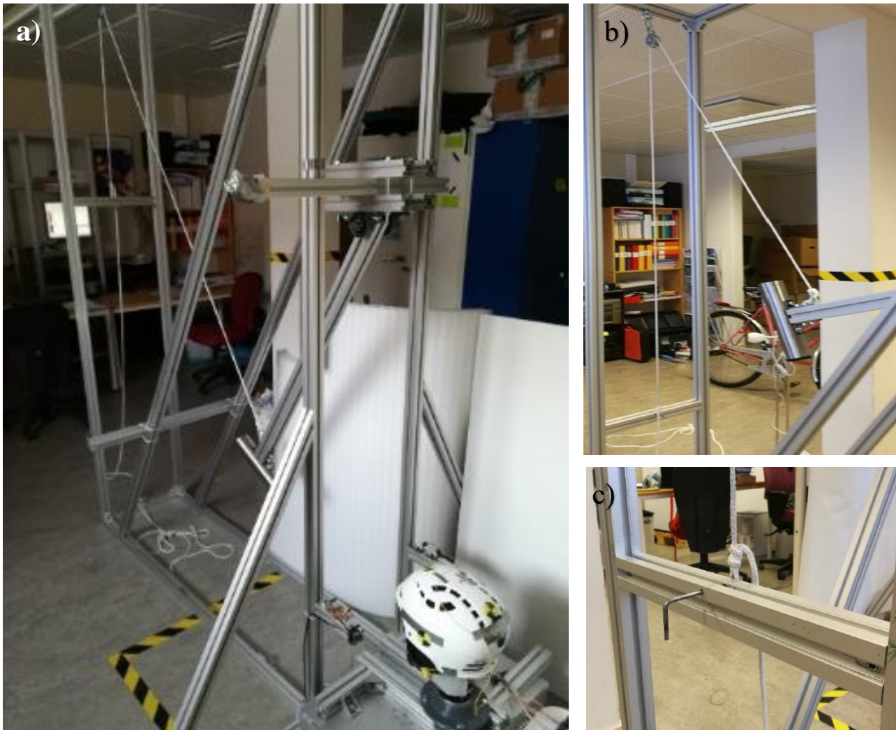
Figure 4.1 (a) Structure. (b) Hammer, rope, pulley and manual trigger. (c) L-shaped manual trigger.
