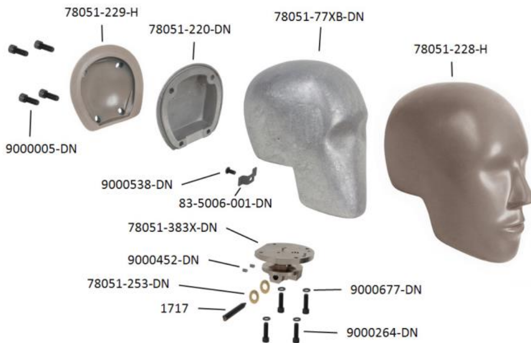
Figure 2.4 Hybrid III 50 th Percentile dummy head composition.
