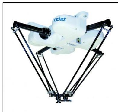
Figura 3.9: Robot Parallelo
