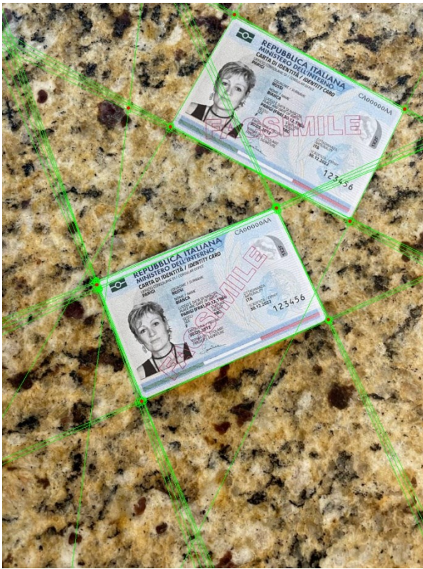
Image 10: Detected lines, intersections and clusters
