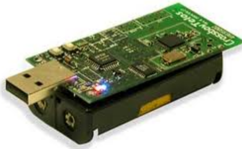
Figura 2.3: A sensor node CrossbowTelos
