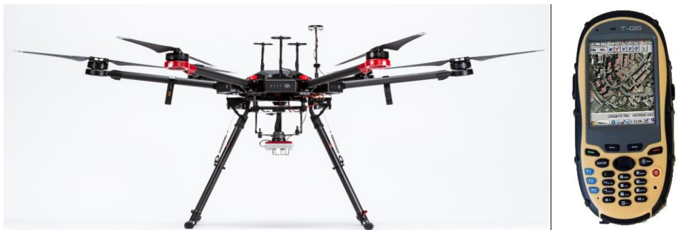
Figure 9: The DJI Matrice 600 drone is utilized for aerial monitoring.( image on the left), Instrument Topcon Hiper pro 2 GPS/GNSS receiver for ground topographic surveys( image on the right)
