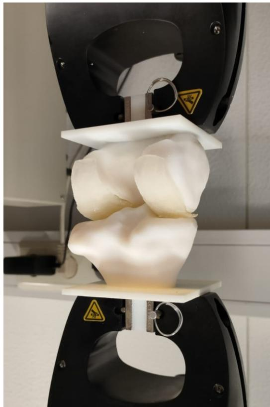
Figure 26. Patient-specific anatomical test setup.
