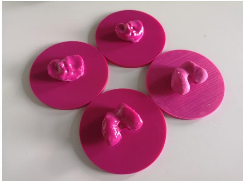
Figure 24. Anatomical supports modified for the patient-specific compression test.
