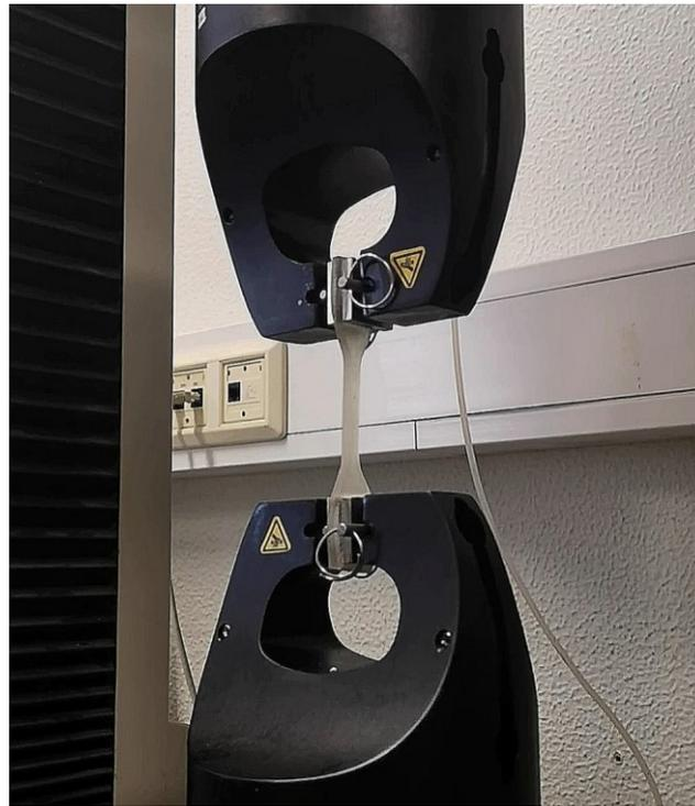
Figure 23. Tensile test on standardized samples.
