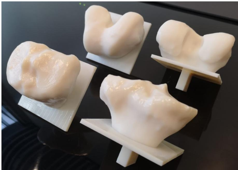
Figure 21. Supports after printing and cleaning.
