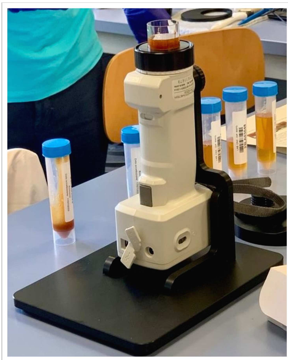
Figure 6.1. Portable VIS spectrophotometer CM-600d, (Konica Minolta Ramsey Sensing, Inc). Picture shows the spectrophotometer fixed in a vertical device, and the cuvette placed on top of the illuminant source. The measurement was conducted in a dark room and the cuvette was rotated by approximately 120^\circ after each scan.
