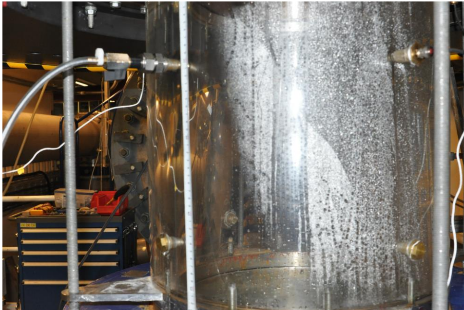
Figure 22- the connection between air injector and draft tube.
