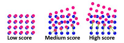
Figure 3.4: Blue = Object cloud. Red World cloud. Three examples of the calculation of the Euclidean Score: the mean value of the green segments
