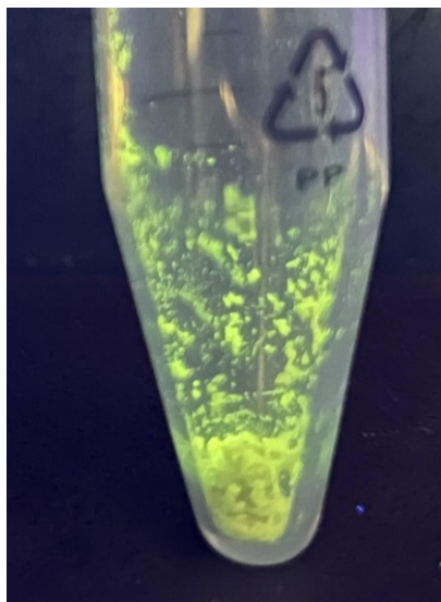
Figure 4.25: Picture of photoactive particles under UV light (365 nm).
