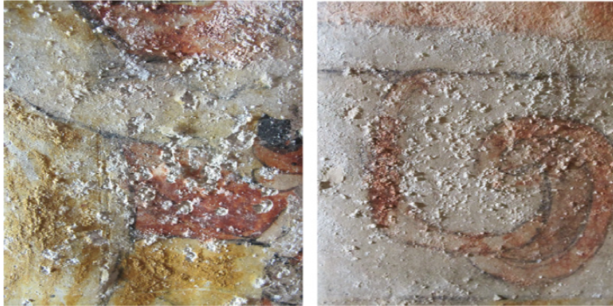
Figure 5.2: Salt efflorescence effects on a pictorial surfaces of site of Ixcaquixtla, Mexico. The detachment of the paint layer due to the mechanical stress of salt crystallization is manifest.[40]
