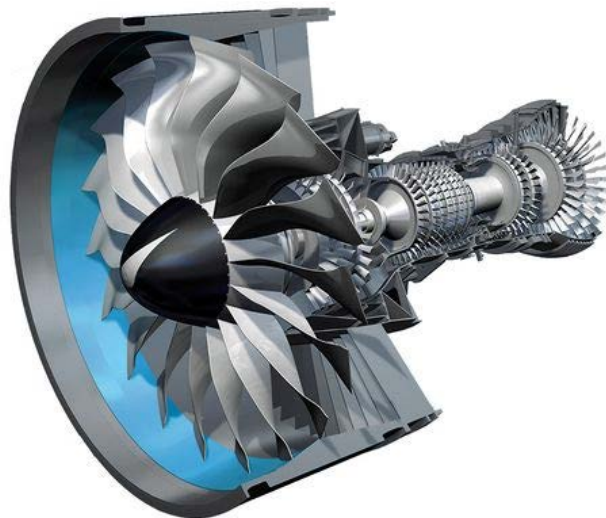
Fig. 3.5: PW1000G engine (MTU, see [24])
