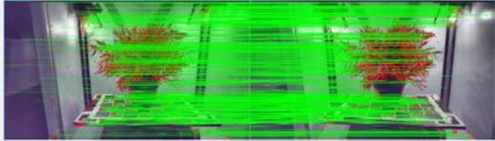
(a) Matches between a pair of images used to perform the reconstruction and the bundle adjustment procedure.
