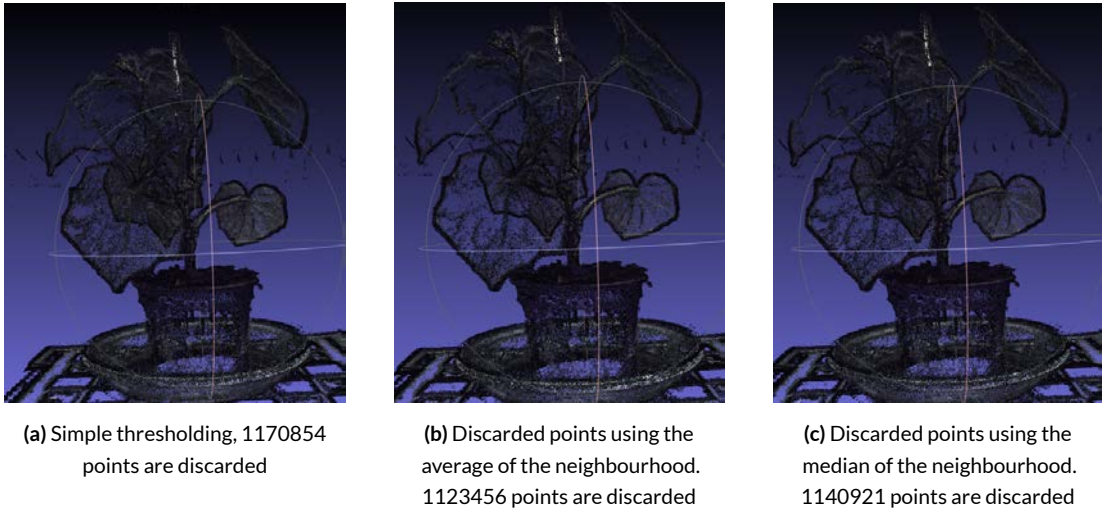
Figure 6.16: Discarded points using NIR threshold of 600 on the simple robust NIR, on the average of the robust NIR of the neighbours and on the median of the robust NIR of the neighbours.
