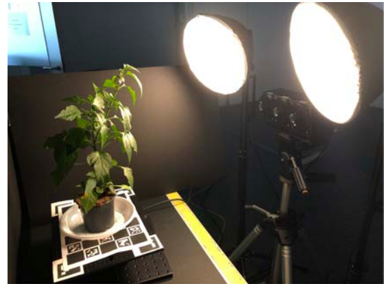
(b) Position of the light sources with respect to the stereo rig
